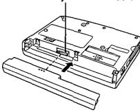
Removing the battery pack
