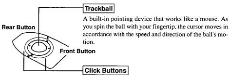
When pressed while the trackball is in use, the buttons select items or perform other operations.
