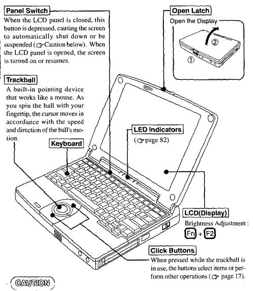
To suspend the screen, [Panel Switch] must be set to [Suspend] ( page 26) in [Panasonic Power Management]. Do not reopen the LCD panel until the power indicator is blinking green. If the LCD panel is reopened before this happens, it may remain suspended and resuming may not be possible. In such cases, close the LCD panel again and wait a few seconds before reopening it.
